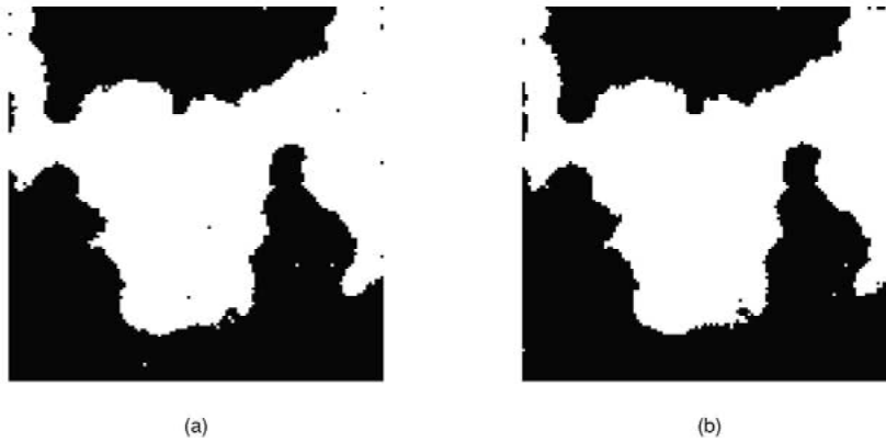
Figure 5. (a) Segmentation with fixed step sizes; (b) Segmentation with decreasing segmentation step sizes.
