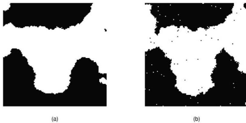
Figure 2. (a) Segmentation with fixed step size; (b) Segmentation with decreasing step size and periodic restart.
